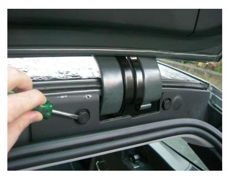
Now the cover is removed. Next step is to remove the plastic plug that holds the lower part of the rightmost wire guide:
