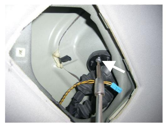
Remove the single screw (torx) which holds the cableloom in place: From here you can retire the cables later...
