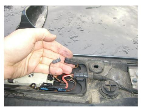
And here is the connector which goes to the glass lid switch:
