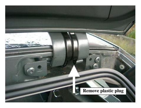
Now, close the boot and open the glass lid (I hope your glass lid switch is still working...). Now you see the upper side of the rightmost wire guide. Unscrew the metal cover with this screw:
